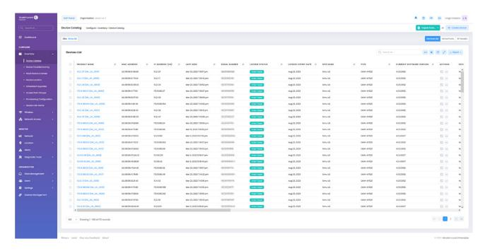
OmniVista Cirrus Catalog provides an overall overview of your network. A single point to control the status of all the network devices: license information, device type, subscription status, connectivity, software release, location, etc.
