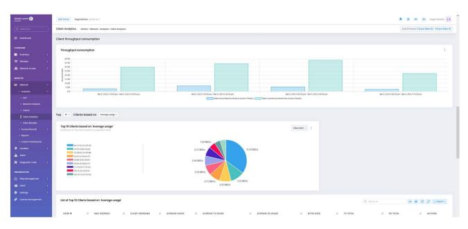
OmniVista Client Analytics shows connected clients' throughput consumption. Monitor and ensure devices receive a fair slice of the bandwidth.
