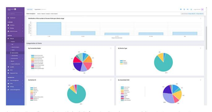
OmniVista Cirrus Client Analytics with detailed information about the connected clients: Device type, Operating System, Wi-Fi standard, SSID most used. IT can monitor and control which devices are allowed in the network.
