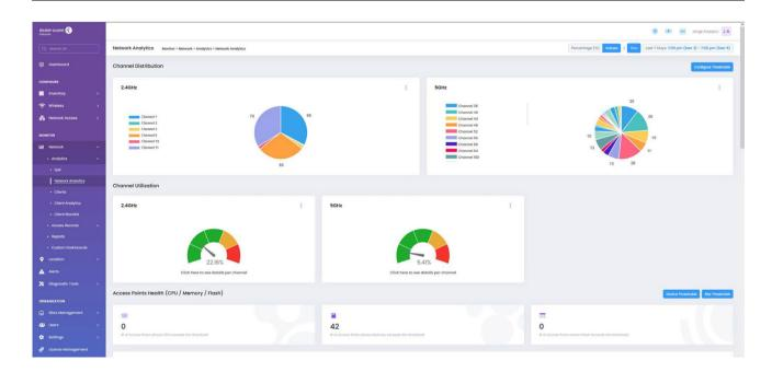
OmniVista Cirrus Network Analytics shows the channel distribution, utilization, and high-level view on Access Points Health. The customizable timeframe allows for monitoring of the WLAN network's health.
