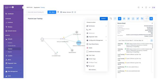
OmniVista Cirrus Topology provides unified WLAN and LAN map layout including device status and graphical network uplink representation
